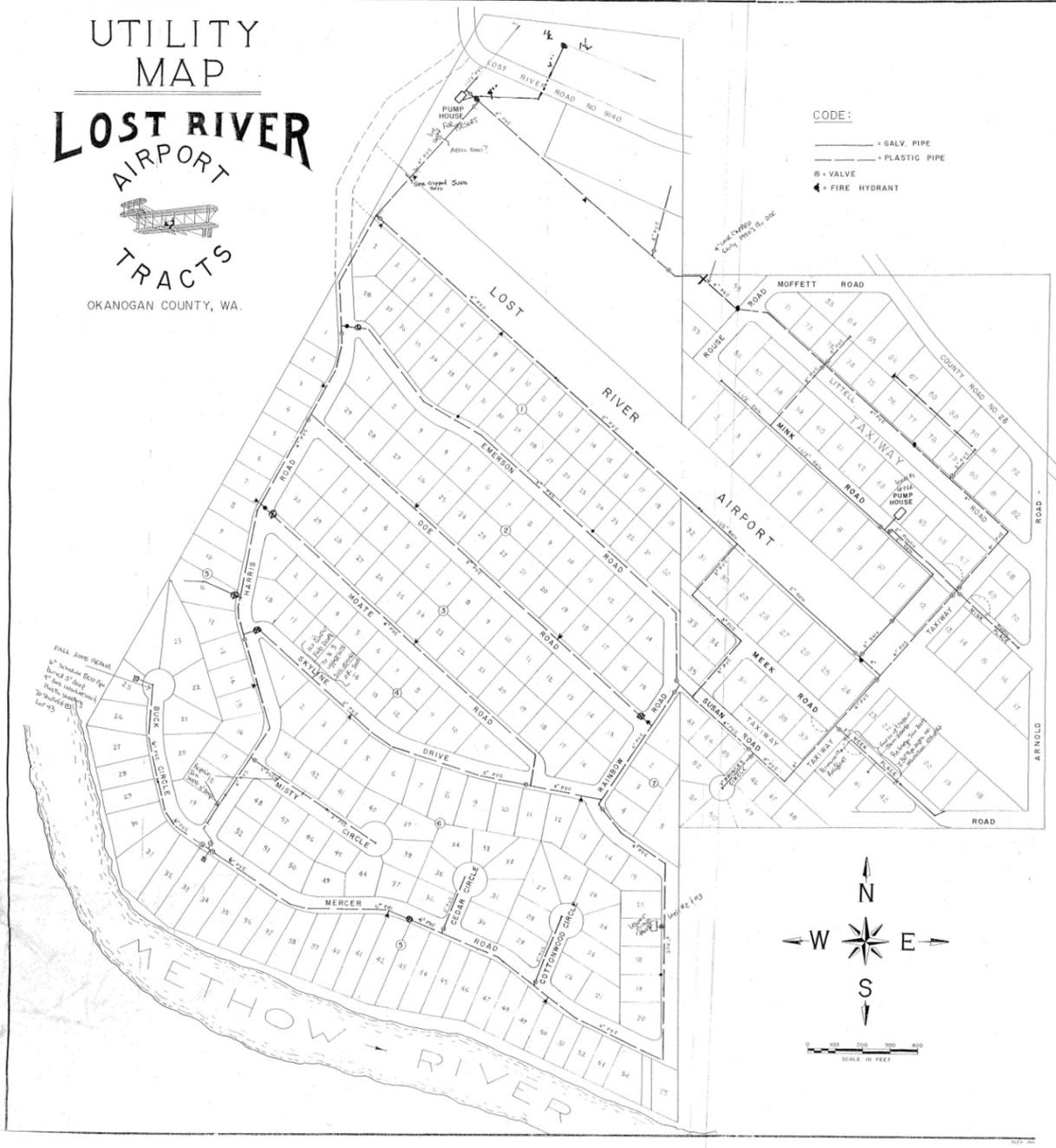
LRAA Utility Map – Showing properties, water mains, shut-off valve locations (digital file available)
